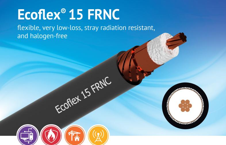
Ecoflex 15 FRNC is a flexible and very low attenuation 50 ohm coaxial cable for the frequency range up to 6 GHz. State-of-the-art production methods and the use of a low attenuation PE-LLC dielectric with a gas content of over 70% enable low attenuation values.
