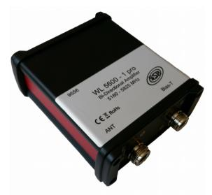
The WL5600-1 is a bidirectional amplifier for the WLAN frequency range 5.18GHz to 5.825GHz. It is equipped with an automatic transmission / reception switch. The gain is min. 25dB. A gain of at least 15 dB is ensured in the receiving direction. The output power can be up to 30dBm (1W).
