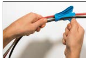
Insert one or more cables into the insertion slot of the HAT applicator tool.
