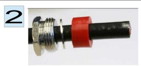
Move the nut, clamping ring and rubber washer over the cable head.
